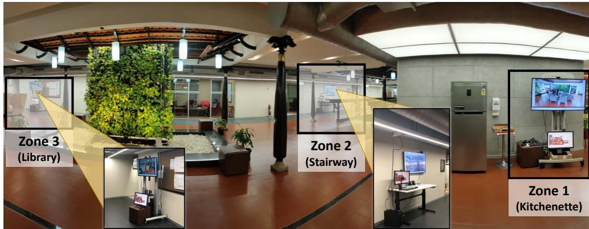
Fig. 1. HyWay deployed in an office workspace. Each setup comprises of a 55 inch display (used to interact with remote users), and a 24 inch display (shows the presence and movement of remote users on the map), wireless mic (Sennheiser SK-100 G3 [22]), speakers (Creative SBS-240 [6]) and powered by a 3.4 GHz processor with 32 GB RAM.
